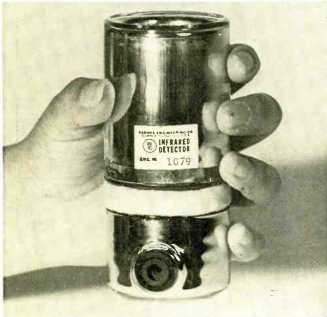
QUANTUM INFRARED DETECTOR. The window visible in the bottom of the Dewar assembly is transparent to infrared wavelengths.
