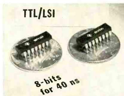
FIG. 4—TI'S NEW SN54/74284 AND SN54/74285 digital ICs.
