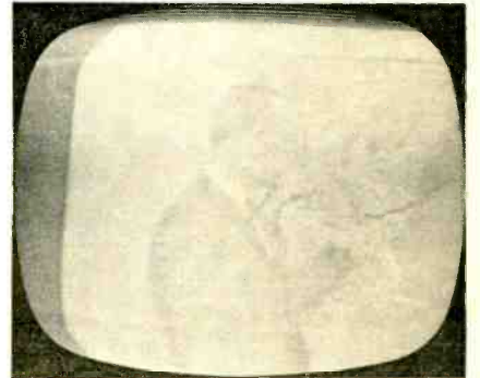
WASHED OUT—TOO MUCH AGC VOLTAGE. RI and i.f. amplifiers are tending to cut off.
