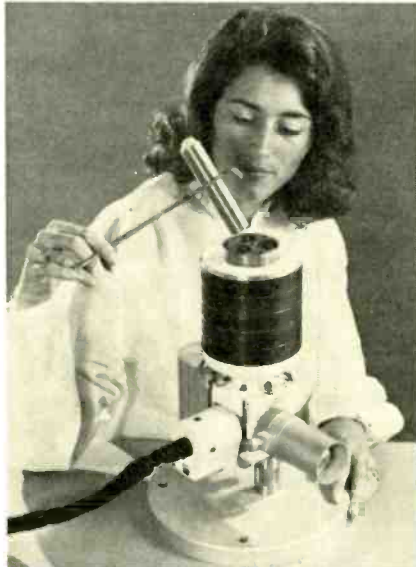
THREE CYLINDERS OF PLUTONIUM 238 provide the energy for the cryogenic 'fridge, which cools things down to more than 300 degrees below zero. The young lady inserting the tubes is Pamela Gleason of Hughes' cryogenic department.
