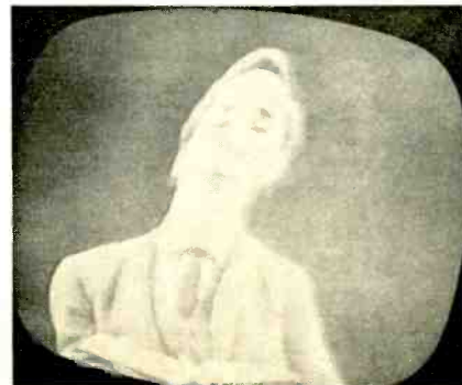
THE PICTURE BENDS—NOT ENOUGH AGC. Video is too strong and beginning to overload.
